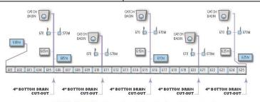
NOTE 1: All half and non-sloped channels have bottom cut outs.
